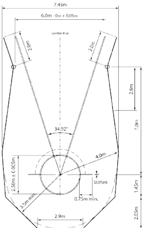
**Figure (b) TR37 - Cage for Hammer and Discus Throw with concentric circles (Discus Throw configuration, with cage dimensions to netting)**
