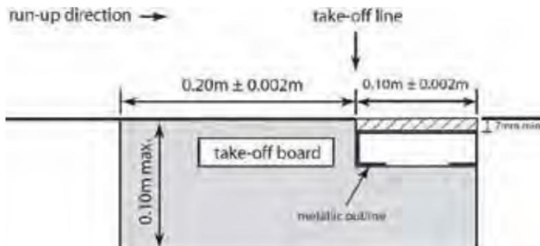
Figure (a1) TR29 - Take-off board with blanking board
